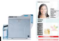
FIPS 201 certified for the personalization of US Government credentials, the Magicard Prima 4 provides a reliable, robust solution for instant issuance in a compact package. Using a retransfer printing process, images are first printed onto a thin film then heat transferred onto the card surface. This produces a high resolution glossy image, printed right over the edge of the card.
